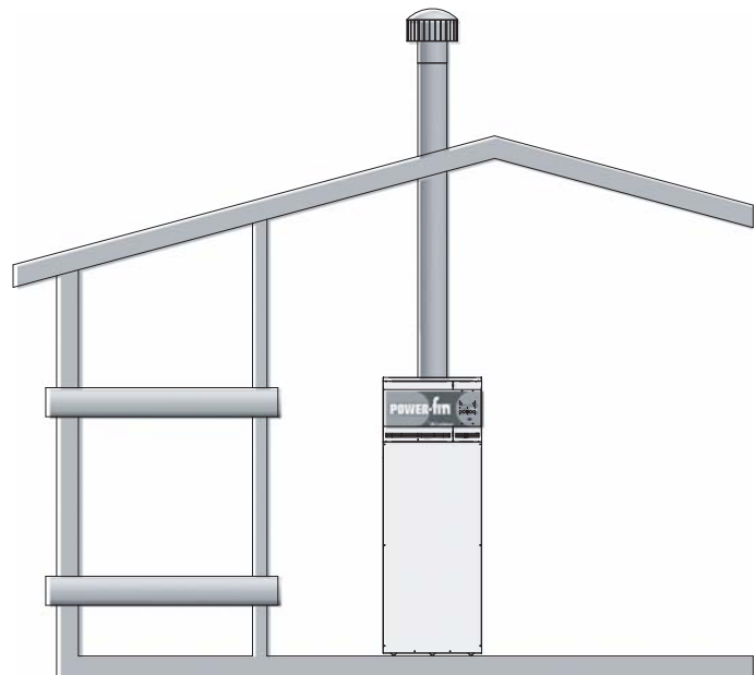
Figure 1-3 Combustion Air Through Ducts
